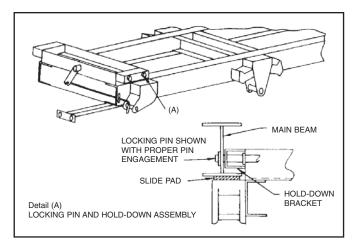
3. Check the pin cage assembly bolts for tightness after each year of service. Re-torque to 380 lb-ft.
